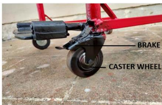
Figure 1: Caster with Brake
