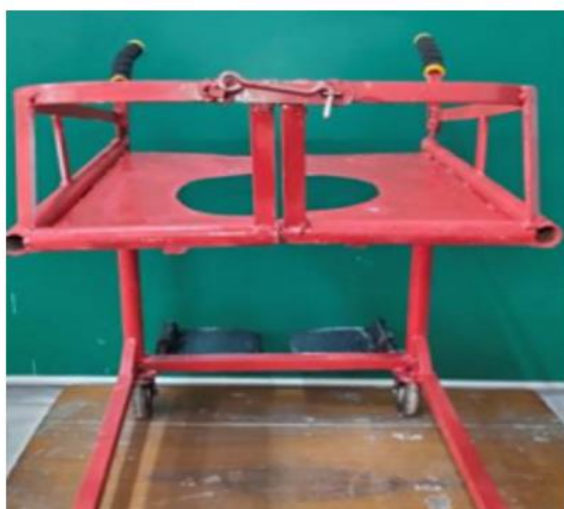
Figure 6: Backrest with Locking Mechanism
