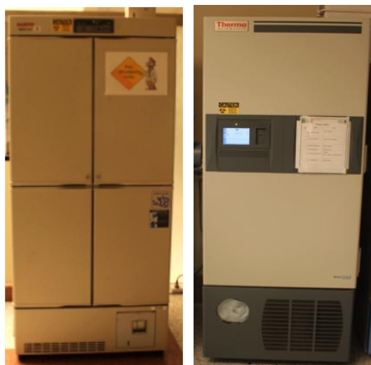
Figure 4: A) A photograph showing the refrigerator used for saliva sample storage at 4°C B) A photograph showing the refrigerator used for saliva sample storage below 20°C
