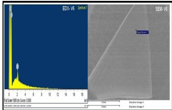
Fig: 10 SEM and EDX Scan of Virgin Plastic Sample (V6)
