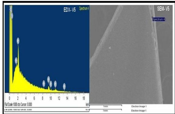
Fig: 9 SEM and EDX Scan of Virgin Plastic Sample (V5)
