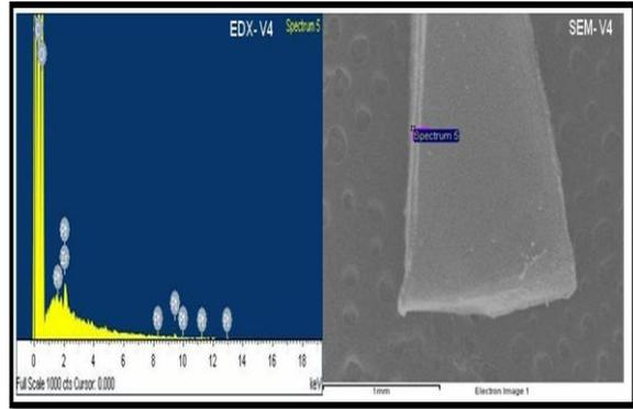
Fig: 8 SEM and EDX Scan of Virgin Plastic Sample (V4)
