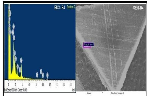
Fig: 18 SEM and EDX Scan of Virgin Plastic Sample (VI4)
