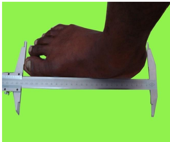
Photo No.2 Photo Showing the Technique Used For the Foot Length Measurement.
